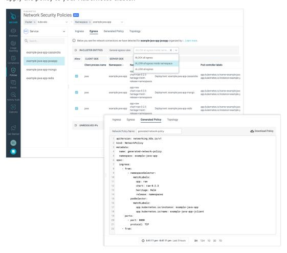
In addition, Sysdig Secure can fingerprint every connection, as well as the processes that are establishing connections. This Audit Tap capability helps cloud teams investigate network activity at a fine-grained level with full visibility into context, including labels. Enterprises subject to regulations, such as NIST and PCI, can leverage this capability along with network segmentation to meet compliance requirements.
